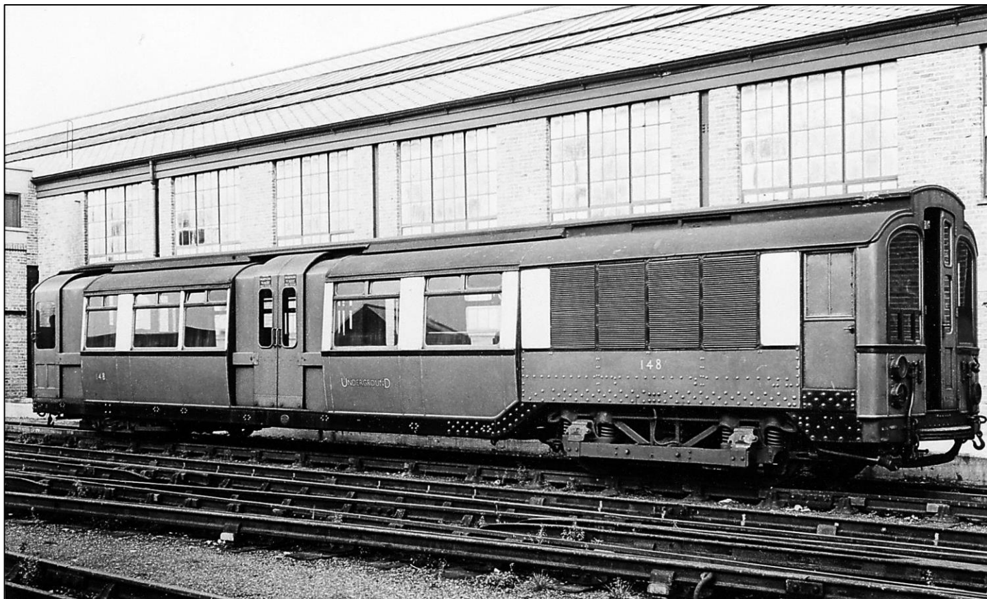
Figure 2: Piccadilly Line motor car No.148 (formerly No.68) waiting to be scrapped in the yard at Acton Works. This car entered service in 1911. Sometime later it was modified and fitted with capstan-operated sliding doors. The end platform was enclosed and fitted with doors and a double doorway was cut into the middle area of the car. The car was fitted with driving controls at the trailing end so that it could be used on the Holborn – Aldwych shuttle service. The car was officially written off on 30 July 1930. The scrapping work had already started when this photo was taken on 8 September 1930. The coupler and tripcock are missing from the front end, having been removed for spares. Photo: LT Museum.
